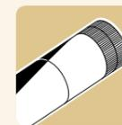
**Balanced Flue** fires vent directly outside through a horizontal co-axial pipe (one pipe within a larger pipe). The outer pipe draws air in from the outside and the inner pipe expels combustion gases. An electricity supply is not required for these products.
