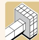
**Powerflue** fires expel the flue gases directly outside the building through the use of an electronically driven fan unit mounted on the external wall. A sophisticated microprocessor monitors performance and automatically shuts off the fire in the unlikely event of operation failure.
